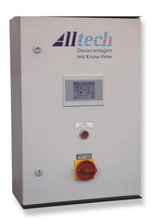
The dosing quantity system, PROCON V4 has been developed for control tasks where the dosing capacity from dosing pumps is controlled either with a guidance signal system or a time control system. When a guide control system is used, switch over is made automatically to a time control system if the signal fails (<2mA).
