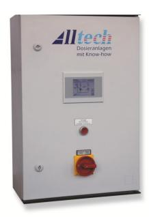
The dosing quantity system, PROCON V3 has been developed for control tasks where the dosing capacity from dosing pumps is controlled either with a guidance signal system or a time control system. When a guide control system is used, switch over is made automatically to a time control system if the signal fails (<2mA).
