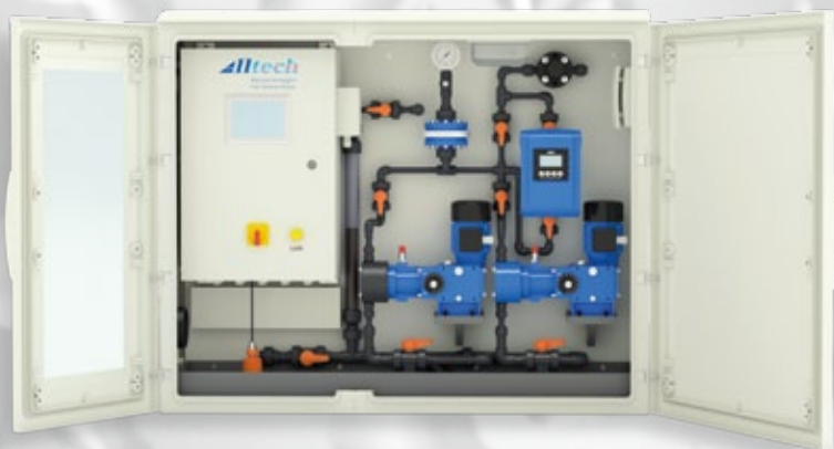
Design configuration, example 1: Dosing unit for polyaluminium chloride (PAC) with robust piston diaphragm dosing pumps model FKM, built-in a protective cabinet, with weather protection roof.
