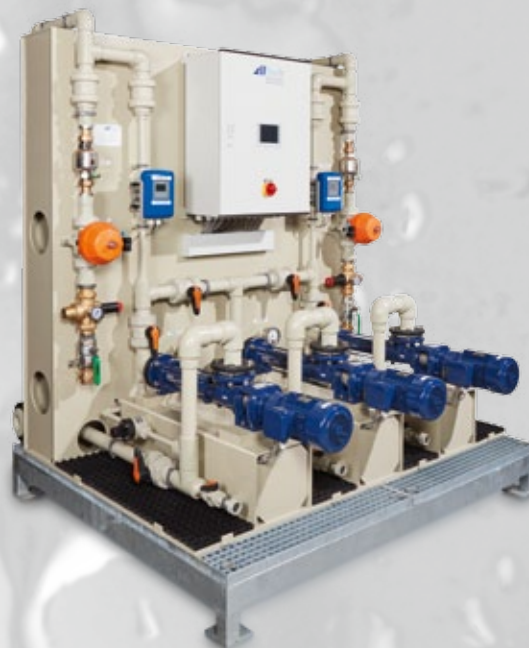
Design configuration, example 2: Dosing skid for floor mounting, suitable for the installation of progressive cavity pumps, for dosing of polyelectrolyte solution. Completely pre-assembled with control cabinet for operation and monitoring.
